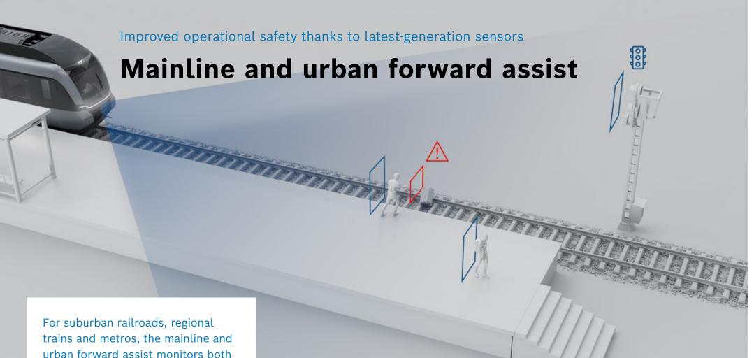
For suburban railroads, regional trains and metros, the mainline and urban forward assist monitors both the area in front of the locomotive and the platform environment on a predictive basis. This helps improve safety at stations and on the open track.
