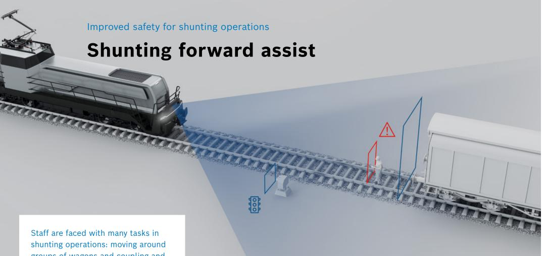
Staff are faced with many tasks in shunting operations: moving around groups of wagons and coupling and uncoupling wagons. At the same time, staff need to pay careful attention to rail activity on parallel tracks. During shunting maneuvers, the shunting forward assist system supports staff and eases the pressure on them by monitoring the area in front of the vehicle on a predictive basis.
